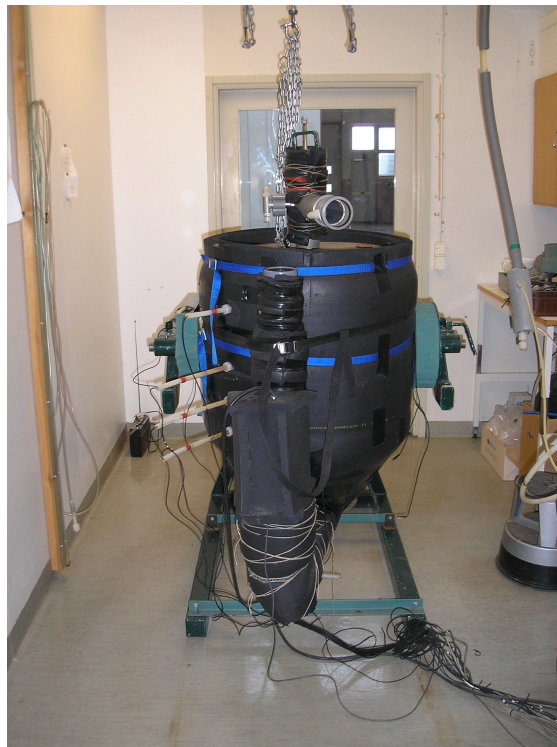
Fig. 6. The laboratory reactor for composting experiments with source-separated organic household waste.
