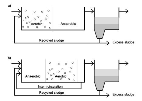
*Figure 6.* The ASP can have two different strategies to ensure efficient removal of nitrogen, a) post- and b) pre-denitrification.
