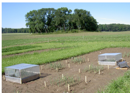
Fig. 2. Pulse labelling of leek with ^{13}\text{C} -enriched carbon dioxide (treatment B) in the experiment at Krusenberg.
