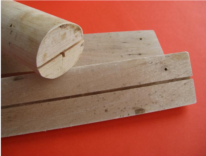
Figure 8. Specially constructed perches providing hiding and mating place for D. gallinae in the experimental study (IV). (Photo: Sofia Holmgren, SLU)
