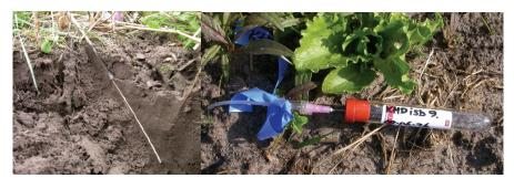
*Figure 5.* Lysimeter installed in the field for sampling soil solution (Papers I, II). Soil has been excavated to show the position of the lysimeter. Photo: Ines Barth and Kerstin Huss-Danell.
