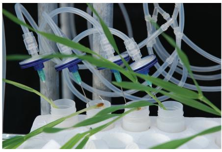
Figure 6. Barley plants in a solution uptake study (Papers II, IV). Tubes for aeration of solution and sterile filters attached to needles are seen in the background.
