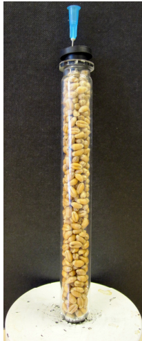
Figure 6. A mini silo containing moist wheat grain with a biopreservation culture and glycerol.
