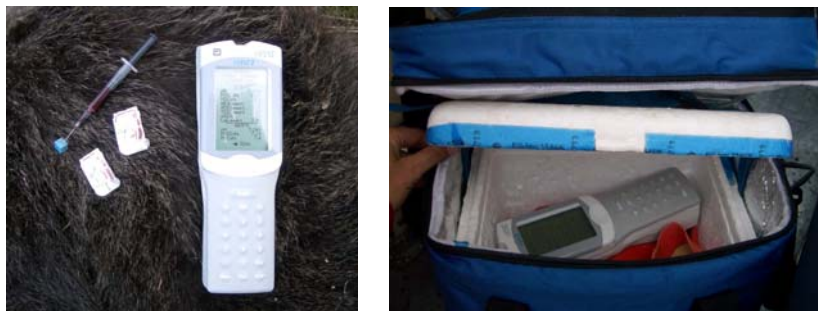
Figure 6. The i-STAT®1 analyser used for field analysis of arterial blood samples (left). Storage of the i-STAT®1 during field work to ensure optimal temperature conditions (right).
