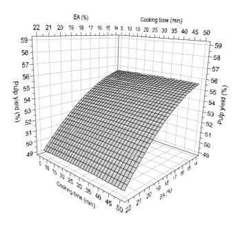
Figure 6a. Screened pulp yield as a function of alkali charge and cooking time for the kraft process. Two stage fractionated RCG.
