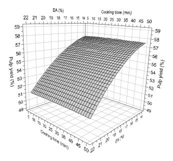
*Figure 6b.* Screened pulp yield as a function of alkali charge and cooking time for the soda-AQ process. Two stage fractionated RCG.
