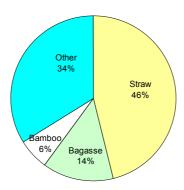
Figure 1. Worldwide use of different non-wood raw materials for pulp production. Data from Paavilainen (1998a).
