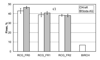
Figure 4. a) drainage, b) fibre length, and c) fines content of RCG pulp produced at different degrees of fractionation with the kraft and soda-AQ processes. RCG\_FR0 indicates no fractionation, RCG\_FR1 fractionation with one stage separation, and RCG\_FR2 fractionation with two-stage separation The error bars indicate  $\pm$  the standard deviation of the measurements.
