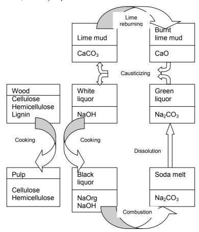
Figure 5. The main steps in the chemical recovery process for a NaOH-based pulping process.
