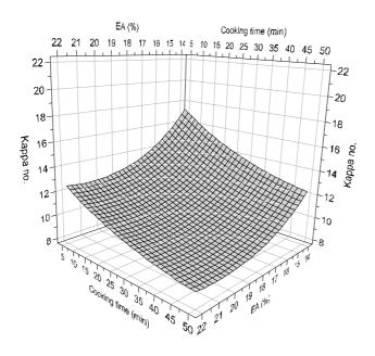
Figure 7a. Kappa number as a function of alkali charge and cooking time for the kraft process. Two-stage fractionated RCG.
