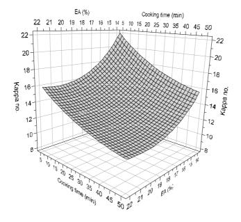
Figure 7b. Kappa number as a function of alkali charge and cooking time for the soda-AQ process. Two-stage fractionated RCG.
