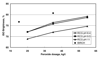
Figure 8. Effect of peroxide dosage on brightness for RCG pulp at different pH levels. Some typical values for birch pulp have been added for comparison.
