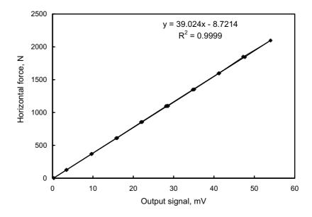
*Fig. 13.* Calibration curve of the octagonal ring sensor with a regression line for output signal and horizontal force (Fx) applied.
