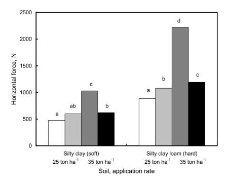
*Fig. 21.* Horizontal forces (Least Significant Means), [N] for tines used at two different soil conditions; for 25 t ha-1:  $\Box$ , double disc (DD) at 5 cm depth;  $\Box$ , small tubulator with sharp tip (TSSh) at 5 cm depth; and for 35 t ha-1:  $\Box$ , double disc (DD) at 8 cm depth;  $\blacksquare$ , medium tubulator with sharp tip (TMSh) at 5 cm depth. Averages with different letters (a-d) within each group are significantly different (probability P < 0.05).
