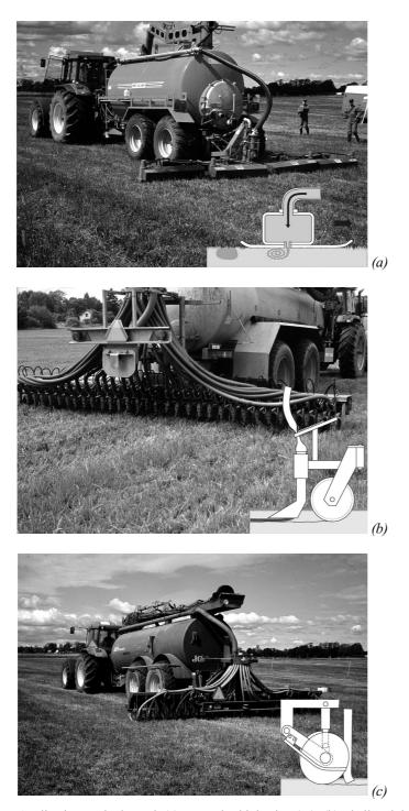
*Fig. 3 a-c.* Application methods used; (a) pressurised injection (PI); (b) shallow injection 1 with open slots; V-shaped disc tine (SIO1); (c) shallow injection 2 with open slots; tine consisting of two angled disc coulters (SIO2).
