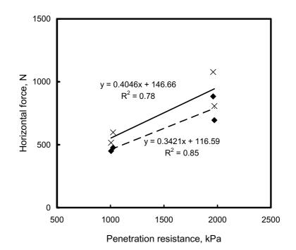
*Fig. 23.* Correlation between soil strength measured with a penetrometer and horizontal forces for the tines:  $\blacklozenge$ , double disc tine (DD);  $\varkappa$ , the small tubulator tine with sharp tip (TSSh) at four soil conditions at 5 cm depth.
