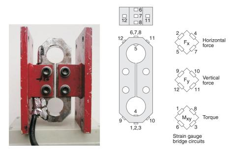
*Fig. 12.* The octagonal ring sensor with the placement of the strain gauges on the steel body and connection in full bridges.
