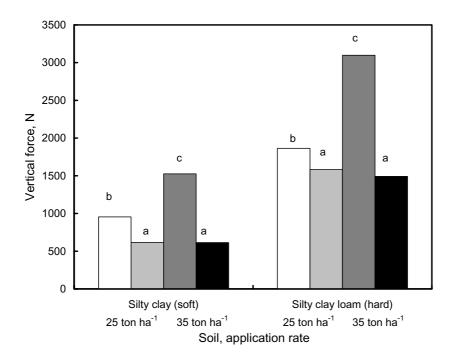
*Fig. 22.* Vertical forces (Least Significant Means), [N] for tines used at two different soil conditions; for 25 t ha-1:  $\Box$ , double disc (DD) at 5 cm depth;  $\Box$ , small tubulator with sharp tip (TSSh) at 5 cm depth; and for 35 t ha-1:  $\Box$ , double disc (DD) at 8 cm depth;  $\Box$ , medium tubulator with sharp tip (TMSh) at 5 cm depth. Averages with different letters (a-d) within each group are significantly different (probability P < 0.05).
