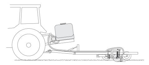
Fig. 11. Trailer with a slurry tanker used in field experiments.
