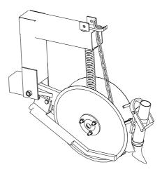
*Fig. 5.* Double disc tine (DD) consisting of two angled disc coulters with diameter of 0.40 m followed by a slurry outlet.
