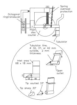
*Fig. 4.* The tubulator with a plain disc coulter followed by a tine consisting of different combinations of three dimensions and two types of tips (6 designs); in addition, the plain disc coulter (PD) was studied on its own.
