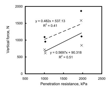
*Fig. 24.* Correlation between soil strength measured with a penetrometer and vertical forces for the tines:  $\blacklozenge$ , double disc tine (DD);  $\aleph$ , the smallest tubulator tine with sharp tip (TSSh) at four soil conditions at 5 cm depth.
