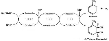
Figure 3.4. Dihydroxylation of toluene to *cis*-toluene dihydrodiol, catalyzed by the three-component TDO system.
