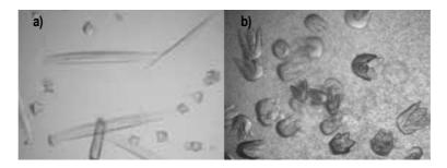
Figure 3.10. Crystals of NBDO. a) Hollow rods (0.05 x 0.05 x 0.3 mm<sup>3</sup>). b) Tulip shaped crystals (0.1 x 0.1 x 0.2 mm<sup>3</sup>).
