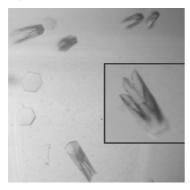
Figure 3.12. Crystals of NBDO. Hexagonal plates  $(0.15 \times 0.15 \times 0.05 \text{ mm}^3)$  and tulip shaped crystals  $(0.15 \times 0.15 \times 0.3 \text{ mm}^3)$ .
