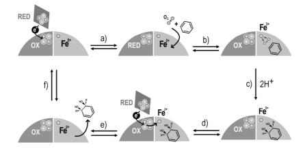
Figure 3.3. Proposed mechanism of dihydroxylation by RDO.
