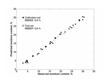
Figure 15. Observed and predicted seed moisture content in calibration (filled circles) and test set (unfilled circles) using a one PLS component model of OSC pretreated spectra (780-2280 nm) from bulk seed samples.
