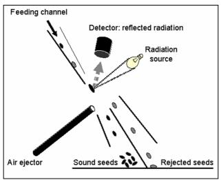
Figure 1. Principle for colour sorting of seeds.
