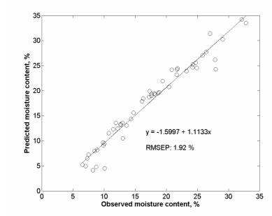
Figure 16. Observed and predicted seed moisture content in test set using a 9 PLS component model based on raw spectra (780-2280 nm) from single seeds.
