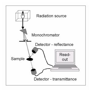
Figure 4. Simplified principle of a NIR instrument.
