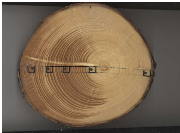
Fig. 4. Sample disc of Norway spruce containing large amounts of severe compression wood. Marked are the small sample areas used for microscopy analysis. The x-ray microdensitometry scanning was conducted along the same radii.
